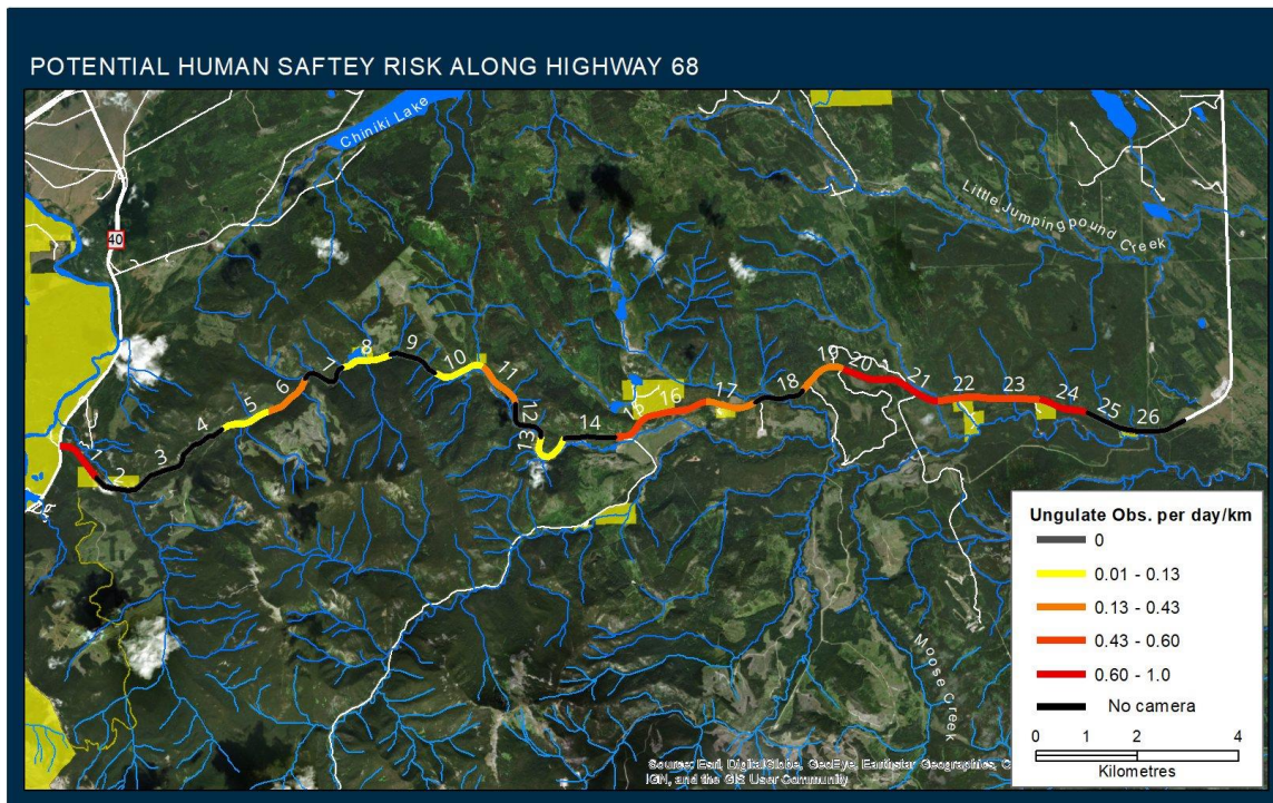
Figure 14: Motorist safety risk per km based on camera detection rates of ungulates
